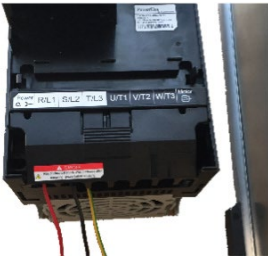
Figure 12: Insulated cable connections
