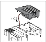
8. Carefully put the fan cover into position in the drive. Make sure that the fan power cable is routed correctly. Push the cover to lock into position.
