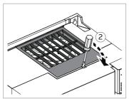
3. Carefully lift the fan cover out of the drive. The fan cover holds the cooling fan.
