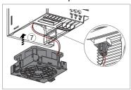
8. Carefully put the fan cover into position in the drive. Make sure that the fan power cable is routed correctly. Push the cover to lock into position.
