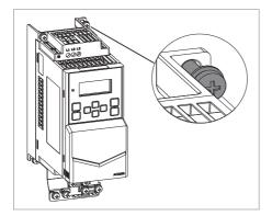
■ To install the drive to a DIN installation rail for frame sizes R0 to R2
